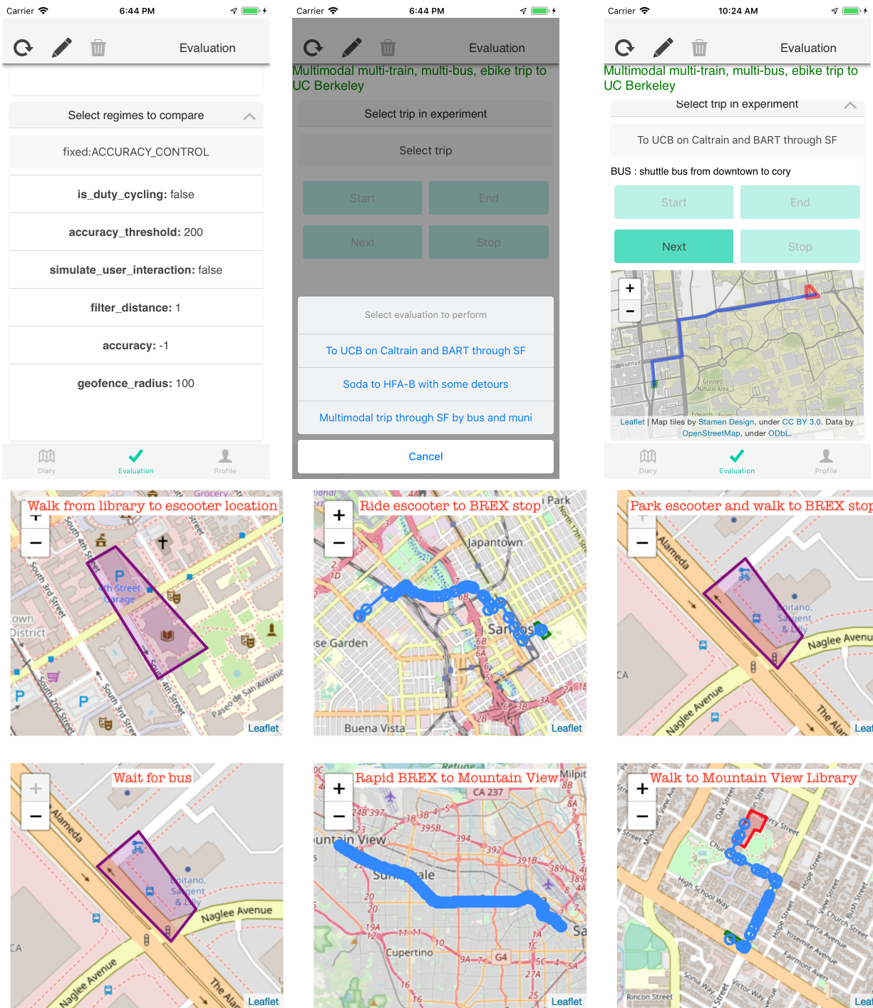
FIGURE 3: Top: Spec components in EM-EVAL-ZEPHYR include configuration, timeline and trip details. Bottom: Sample spec for a multi-modal trip, including transfers and waits for public transit.
